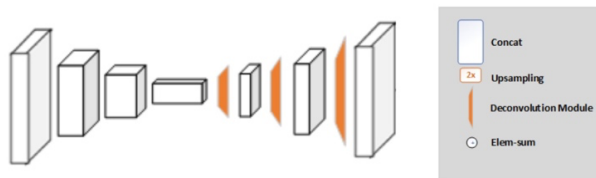
Figure 2. Visualization of ResNet Model Architecture showing different convolutional layers (Xiao et al., 2018)
