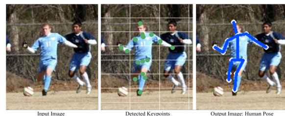
Figure 1. Human pose estimation using a ResNet-based machine learning model. The input frame (left) is processed to predict human body keypoints (center, green), which are subsequently structured into a kinematic skeleton (right, blue), effectively visualizing the estimated human pose.
