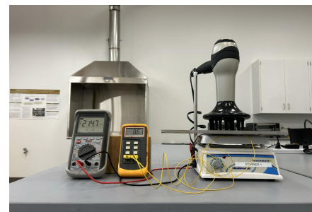
Figure 3. An experimental setting from a single TEG. TEG was placed between hot plate and metal plate, and then wired with a thermometer and multimeter to measure the temperature and voltage respectively.
