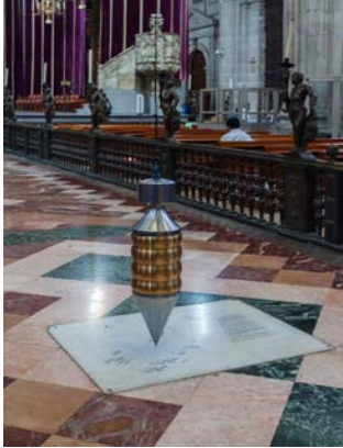
Figure 2. A spring pendulum that is suspended three stories above from the roof of the Cathedral Metropolitana in Mexico City (Photo Credit: Diego Delso, License: https://creativecommons.org/licenses/by-sa/3.0/ ) (Wikiwand).
