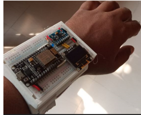
Figure 2: Example of a tremor monitor system hooked up to a patient’s wrist.
