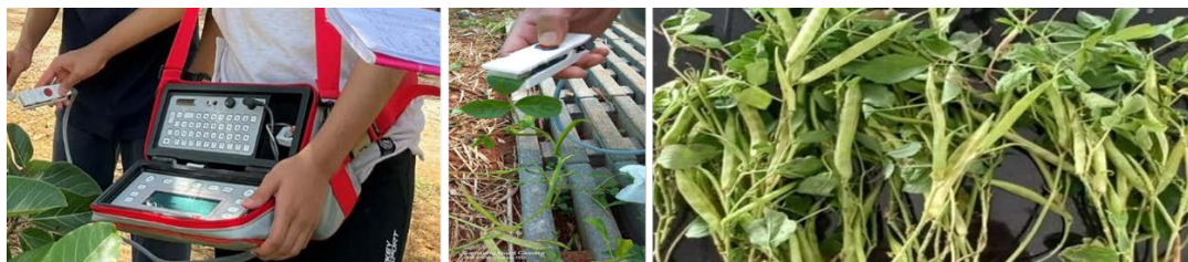
Figure 13. Leaf Porometer (AP4 leaf porometer, Delta-T Devices, UK) used during the experiment (measurement of stomatal conductance)
