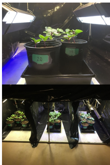
Figure 3: Image of trial 1 light setup where UVA light is 25 cm and UVB light is 15 cm away.
